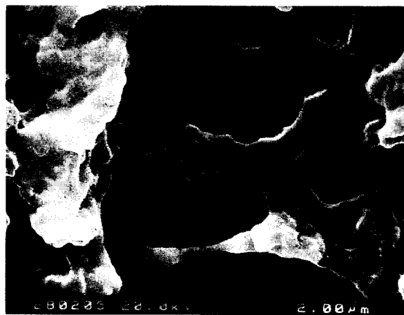
Figure 3 SEM micrograph of a sample formed by vacuum drying at room temperature; hexanediol dichloride content: 1.48 wt%; polymer content in the suspension: 8.0 wt%
